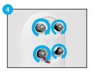
Tightly secure each **bolt** with the **washers and nuts**.
