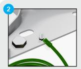
For pole-mounted antennas, attach the 10 AWG or thicker ground wire to your metal pole.
