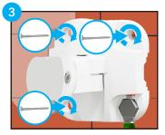
Fully secure your FlexMount with the remaining **screws**.
