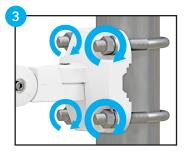
Secure each **U-bolt** with its **washers** and **nuts**.
