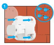
If necessary, drill pilot holes and insert wall anchors.
