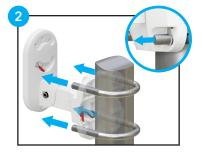
Insert the **U-bolts** through the mount's integrated **ground wire**.
