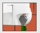
For wall mounted antennas, attach the 10 AWG or thicker ground wire to the grounded FlexMount screw.
