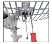
8. If you need to cross-polarize the antenna, loosen the screw on the rotational mount. Tighten again afterwards
