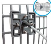
4. Slide the feedhorn's pigtail through the center hole of the grid, and insert 4 bolts through the feedhorn and grid
