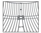
**1.** Bring the two halves together with the tabs overlapping.
