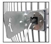
**5.** Place the rotational L-bracket over the bolts and pigtail. Tighten the feedhorn, grid and bracket together with 4 nuts.
